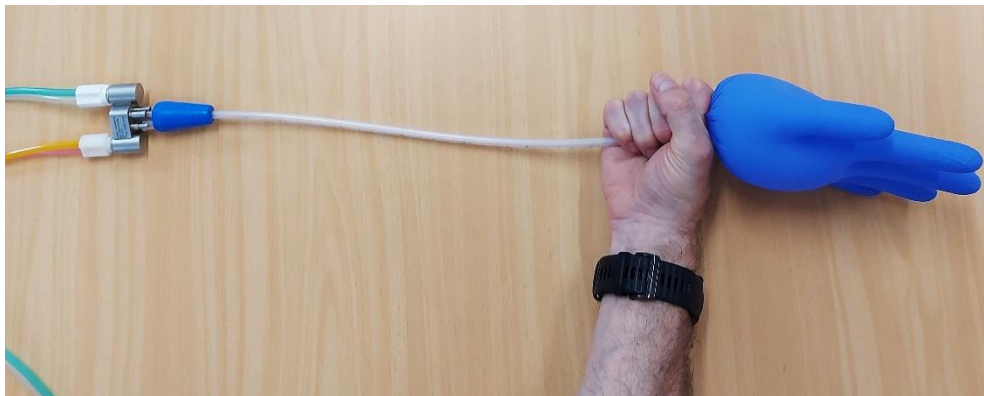
Figure 6: Pressure test. Ventilation is running. Glove inflates.
