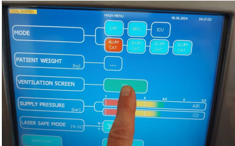
Figure 3: Mode "4LUM CAT" and Ventilation Screen OK
